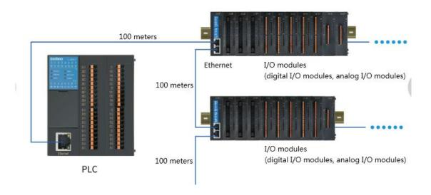
The communication bus protocol adopts the standard EtherNet/IP communication bus, which can easily realize barrier-free connection with EtherNet/IP PLC or industrial computer. The communication interface mode is 2 RJ45 100M Ethernet interfaces, which realize the port switching function internally, and multiple slave stations can be easily cascaded without adding a switch.
