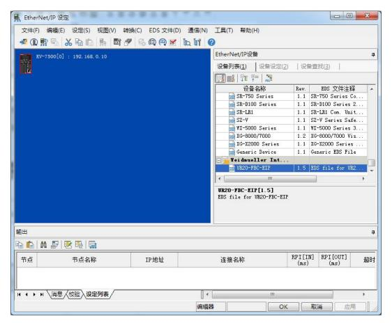
(2) Double-click UR20-FBC-EIP to add a device, set the node address and IP
