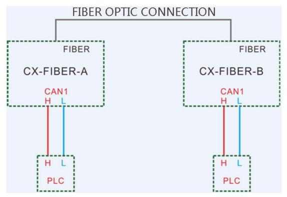
2. CAN communication between PLC and PLC - two CANs can be used simultaneously or independently
