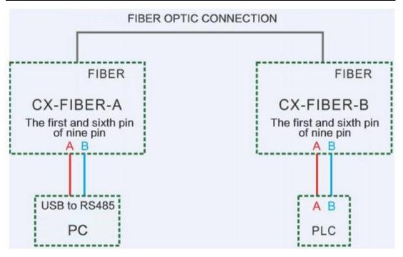
4. Between PLC and PLC or between PLC and computer can also communicate via fiber to RS232. (MODBUS protocol and programming port protocol)
