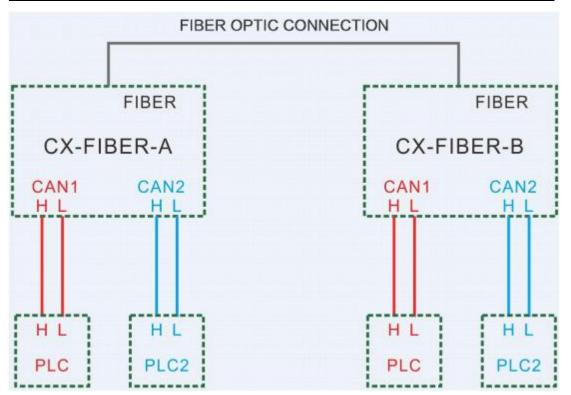
3. Between PLC and PLC or between PLC and computer can also communicate via fiber to RS485. (MODBUS protocol and programming port protocol)
