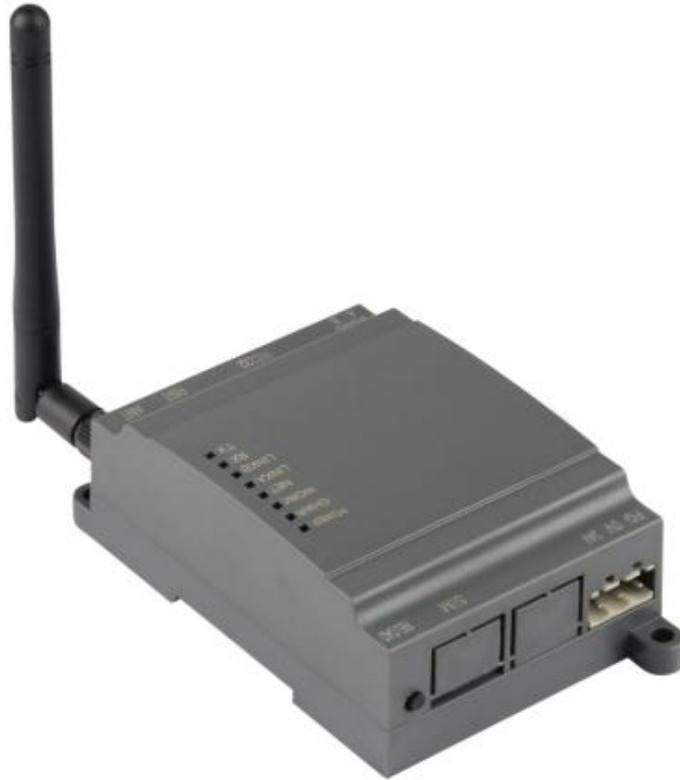
CX-4G is a small, feature-rich GPRS transparent transmission module for Mobile, China Unicom, Telecommunications 4G and Mobile, China Unicom 3G and 2G network standard.
