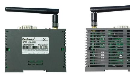
CM-GPRS is a wireless communication module adopts transparent transmission combined with GPRS. It can realize the connection between automatic system and GPRS and GSM used together with Coolmay PLC. Programming, diagnosing, uploading and downloading in a remote distance can be achieved through programming software. Cellphone users can control PLC through SMS messages. CM-GPRS can be particularly applied to distributed remote monitoring system.
